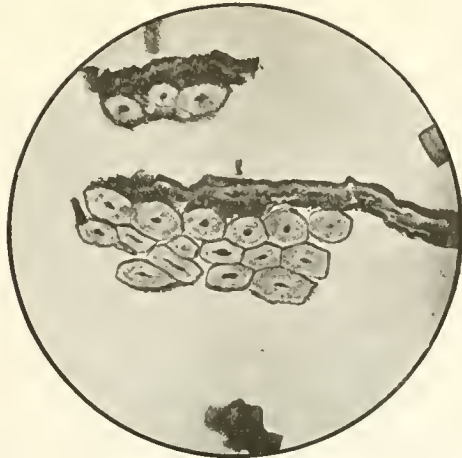
Fig. 21. Transverse section of a typical flax-fibre from middle of stem (Pernau-flax) in zinc chloride iodide. Mag. 300x.
